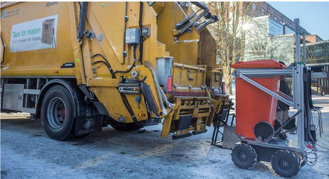
When it is time to begin waste collection, the driver of the refuse truck presses a button. This starts the robot and the drone simultaneously lifts from the roof of the truck. Flying through alleyways, the drone quickly finds the location of the refuse bins and communicates their positions to the robot. This is followed by automatic waste collection and emptying by the robot. In the cab, the driver is able to monitor the exact location of the [robot](#) and the emptying process.
