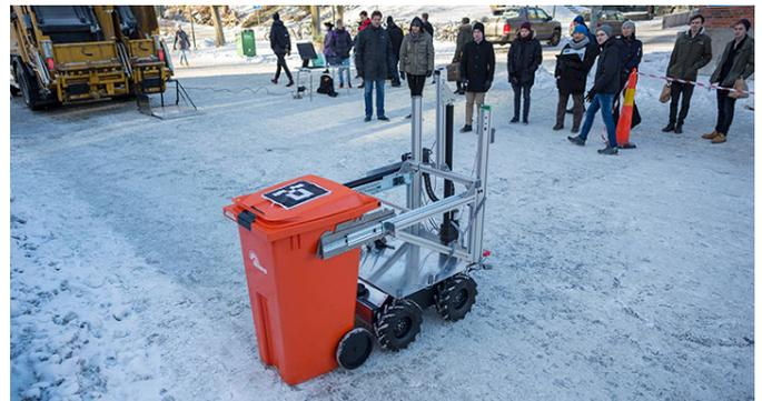
At Chalmers University of Technology, three student groups were involved in developing systems for bin detection, safe emptying, and overall system coordination.
