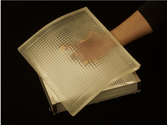
Columbia Engineering researchers have developed a novel sheet camera that can be wrapped around everyday objects to capture images that cannot be taken with one or more conventional cameras. They designed and fabricated a flexible lens array that adapts its optical properties when the sheet camera is bent. This optical adaptation enables the sheet camera to produce high quality images over a wide range of sheet deformations. Credit: Columbia Computer Vision Laboratory, 2016/Columbia Engineering
