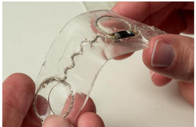
Researchers at The Ohio State University are developing embroidered antennas and circuits with 0.1 mm precision -- the perfect size to integrate electronic components such as sensors and computer memory devices into clothing. They are also exploring other uses for the technology, including this flexible circuit that contains an RFID chip. Credit: Jo McCulty, courtesy of The Ohio State University
