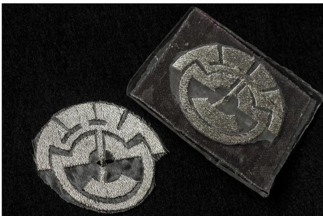
Researchers at The Ohio State University are developing embroidered antennas and circuits with 0.1 mm precision--the perfect size to integrate electronic components such as sensors and computer memory devices into clothing. This antenna features interlocking geometric shapes that provide broadband signal transmission. Credit: Jo McCulty, courtesy of The Ohio State University.
