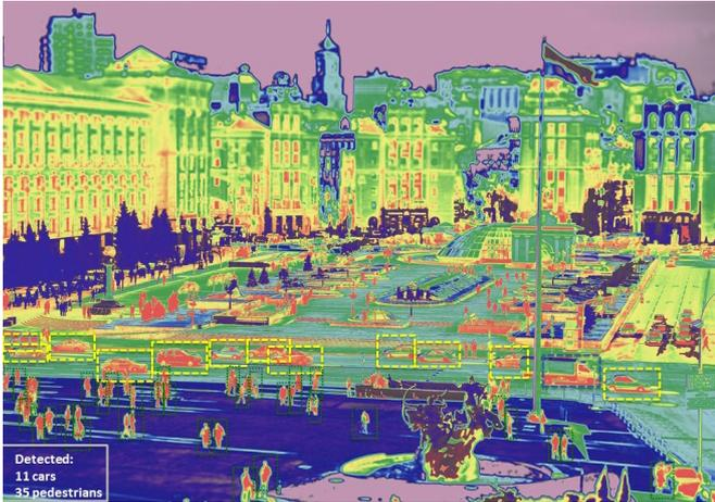
Thermal imaging and machine vision applied to pedestrian and vehicle counting to understand traffic flows. Thermal imaging performs well in various weather and light conditions, in addition to being able to easily differentiate the background from live subjects through heat signatures.
