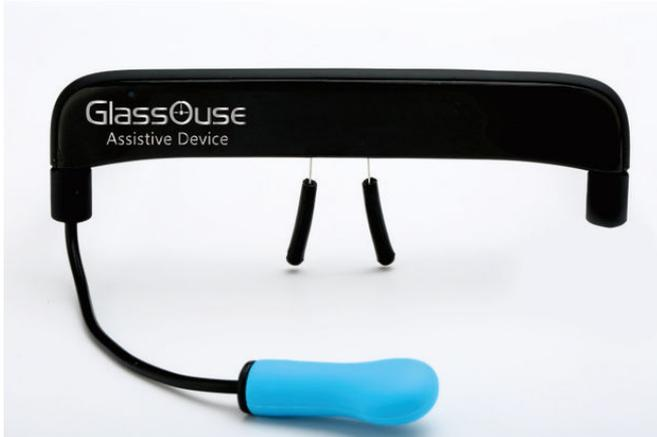
(Tech Xplore)—A team led by designer Mehmet Nemo Turker has posted an Indiegogo project for a head-mounted device called GlassOuse (Glass Mouse)—it is meant to allow disabled people to use a computer or handheld device by converting head movements into control mechanisms.
