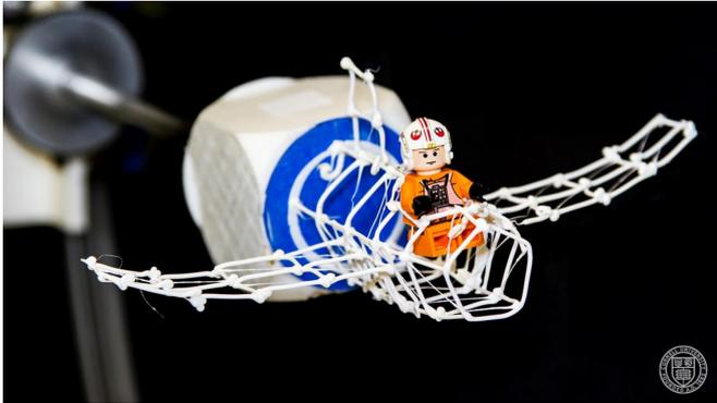
This wire frame prototype of a toy aircraft was printed in just 10 minutes, including testing for correct fit, and modified during printing to create the cockpit. The file was updated in the process, and could be used to print a finished model. Credit: Cornell University
