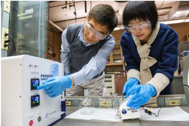
Principal chemical engineer Jie Li, left, and postdoctoral researcher Alina Yan create coated nanoparticles in a continuous flow reactor. Nanoparticles are key to an ongoing effort at Argonne to create more efficient window films. Credit: Argonne National Laboratory
