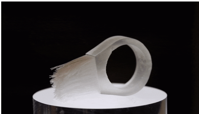
The researchers attached the 3-D printed hairs to a ring. Credit: Massachusetts Institute of Technology
