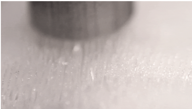
Vibrations cause a piece of metal to move across the 3-D printed hairs. Credit: Massachusetts Institute of Technology
