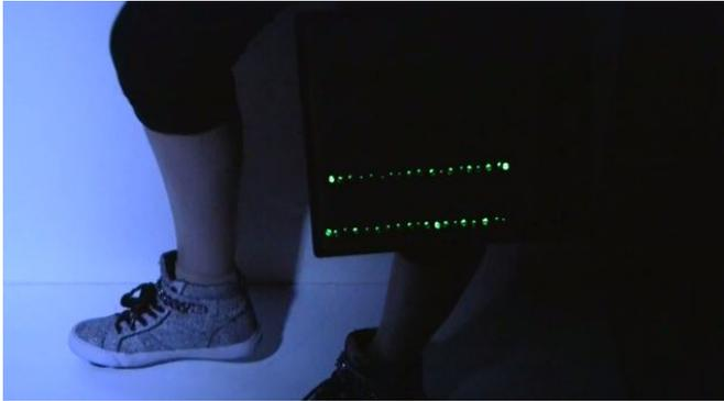
(Tech Xplore)—A combined team of researchers with members from several institutions in China and the Georgia Institute of Technology, has developed a flexible nanogenerator that harnesses the energy from moving body parts and uses it to run electronic devices. In their paper published in the journal *Science Advances*, the team describes their new device, how they made it bendable, and the ways they believe it might be used.
