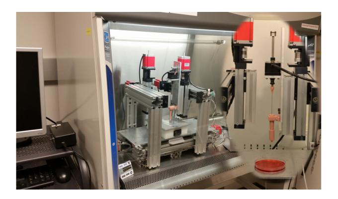
A multiarmed bioprinter used to 3-D print cartilage. A special nozzle for printing bioink composed of strands of cartilage can be seen. Credit: Ozbolat, Penn State
