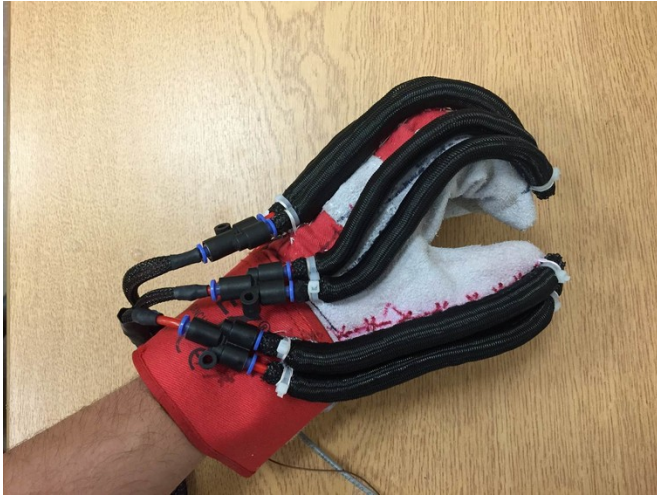
Prototype soft exoskeleton glove. Credit: Steve Davis, Author provided
