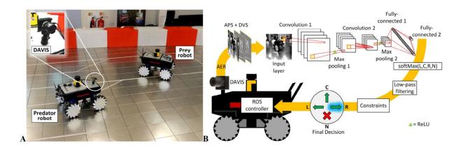
A: Summit XL predator (left) chasing the prey (right) in the robot arena of the University of Ulster, Londonderry. B: overall closed-loop system: the DAVIS sensor generates APS and DVS data which is alternately fed to the 4C5-R-2S-4C5-R-2S-40F-R-4F convolutional neural network. The results are filtered and the final decision is used in conjunction with the laser scanner output to control the Summit XL behavior in the ROS controller. Credit: arXiv:1606.09433 [cs.RO]
