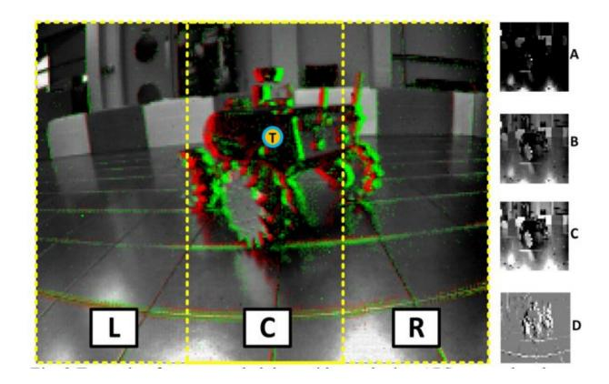
Example of raw recorded data with overlaying APS gray value data and DVS data (red are OFF events, green are ON events). The field of view is divided into the three regions and the target is labelled. A, B and C are the extracted 36 x 36 APS frames with falsely created exposures. D is a subsampled DVS histogram. Credit: arXiv:1606.09433 [cs.RO]
