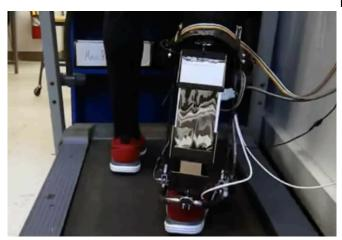
The electroadhesive clutch is a slim, lightweight, and energy-efficient alternative to conventional clutches in robotics. Credit: Carnegie Mellon University Mechanical Engineering
