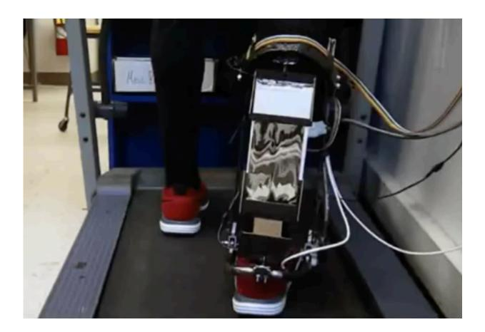
The electroadhesive clutch is a slim, lightweight, and energy-efficient alternative to conventional clutches in robotics. Credit: Carnegie Mellon University Mechanical Engineering
