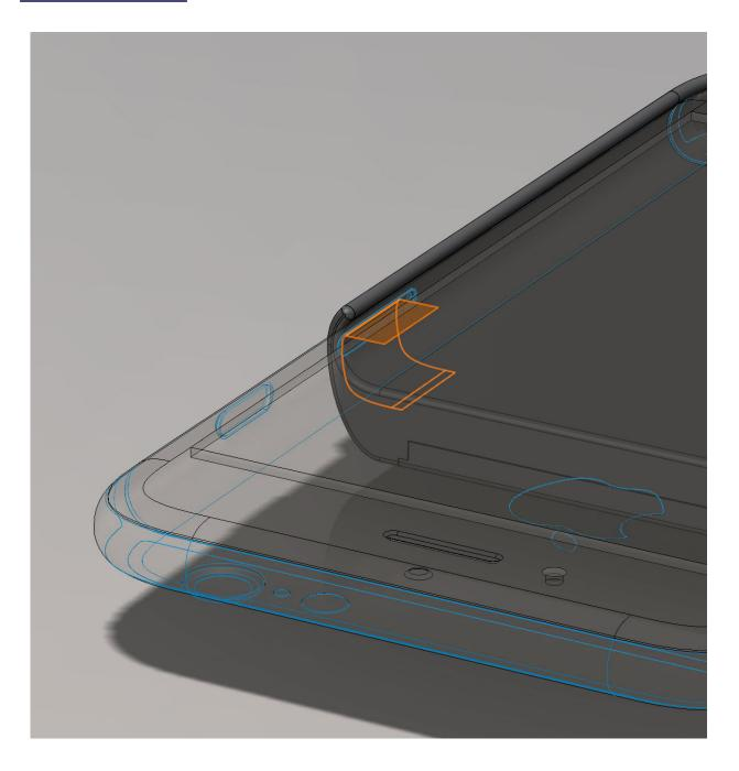
The orange highlighted part is a proposed FPC which exits via the SIM card port and routes signals from the modified iPhone6 mainboard to the introspection engine's electronics. Credit: pubpub.org
