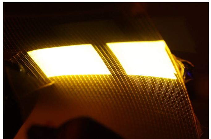
Ultra-flexible, lightweight light-emitting textile. Credit: Lanz et al. ©2016 IOP Publishing Ltd
