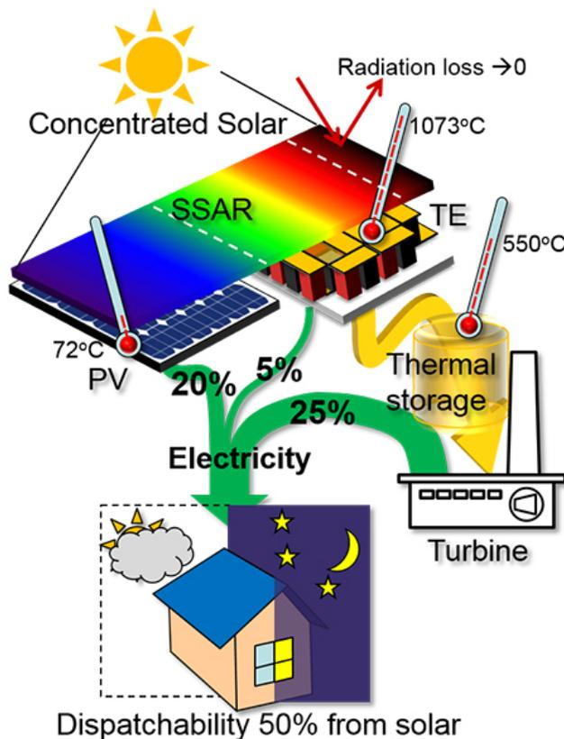
This schematic depicts a new concept that could bring highly efficient solar power by combining three types of technologies that convert different parts of the light spectrum and also store energy for use after sundown. Credit: Purdue University image/Peter Bermel
