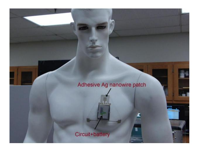
The new sensor, which tracks an individual's skin hydration in real time, can be incorporated into a wearable patch. Credit: Shanshan Yao
