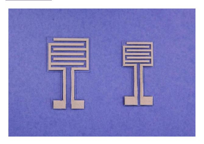
The hydration sensors consist of two electrodes made of an elastic polymer composite that contains conductive silver nanowires. Credit: North Carolina State University
