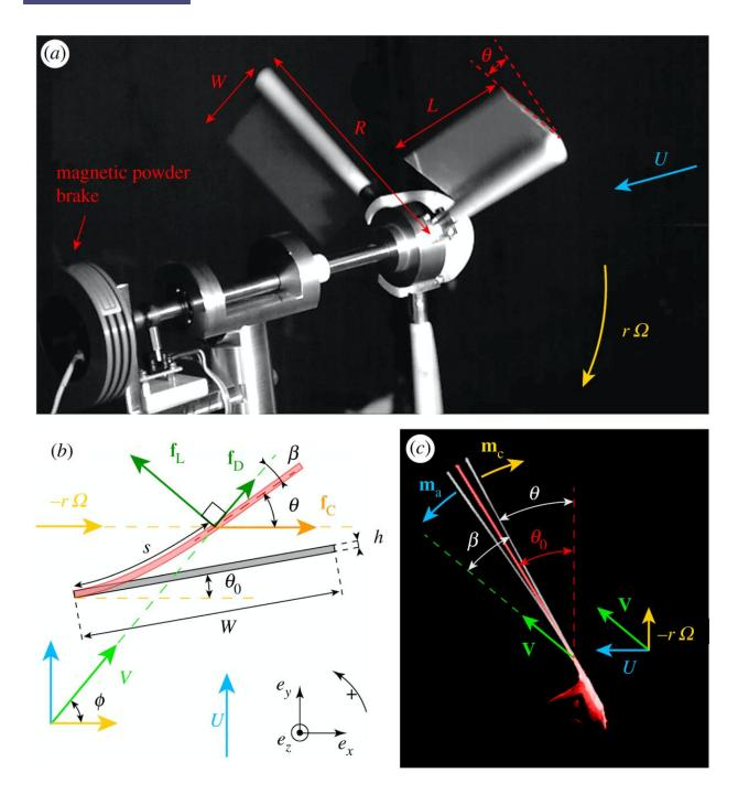
(a) Three-bladed turbine model used in this work. (b) Sketch of a blade section in the rotating frame of reference, showing symbols and notation. During the operating regime, the blade is subjected to the aerodynamic force (decomposed into lift fL and drag fD), which tends to fold the blade through the action of the torque ma, and the centrifugal force fC, which conversely tends to align the blade with the rotation plane due to the torque mc exerted in the opposite
