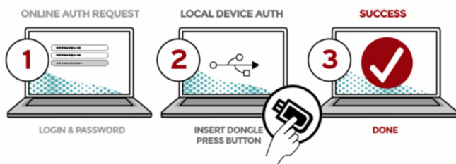
How a login works with a physical key. Credit: FIDO Alliance
