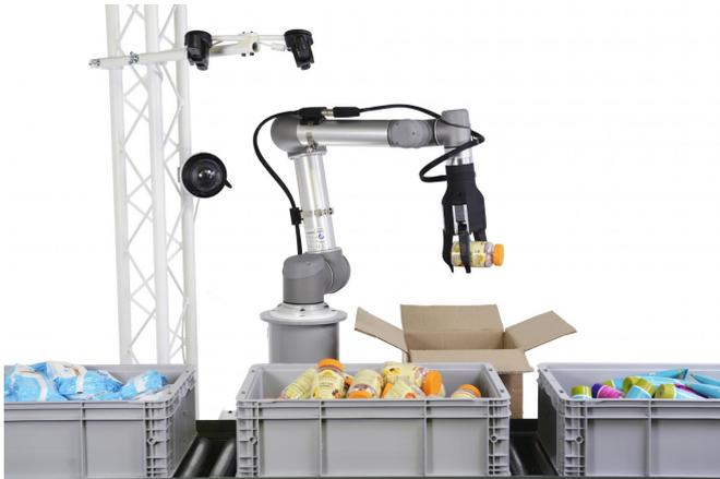
(Tech Xplore)—RightHand Robotics has introduced RightPick. This is a combined hardware and software solution that handles the key task of picking individual items, or "piece-picking."
