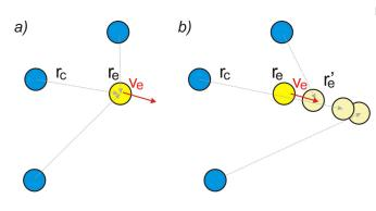
The chasers (blue) are chasing (a) the current position of the escaper (yellow) and (b) its position predicted. Credit: *New Journal of Physics* (2017). DOI: 10.1088/1367-2630/aa69e7
