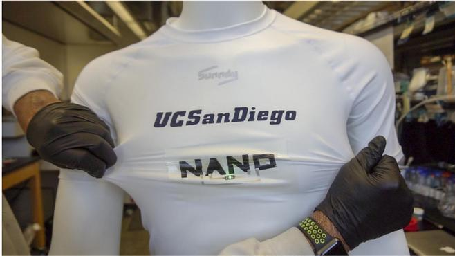
The stretchable batteries were printed on fabric for this demonstration. They make up the word NANO on the shirt and are powering a green LED that is lit in this picture. Credit: Jacobs School of Engineering/UC San Diego
