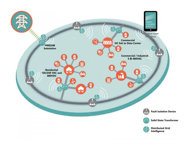
This diagram shows how solid-state transformers could be incorporated into a smart grid power system. Credit: FREEDM Systems Center, North Carolina State University
