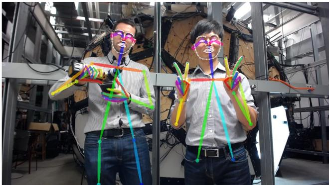
Carnegie Mellon University researchers have developed methods to detect the body pose, including facial expressions and hand positions, of multiple individuals. This enables computers to not only identify parts of the body, but to understand how they are moving and positioned. Credit: Carnegie Mellon University
