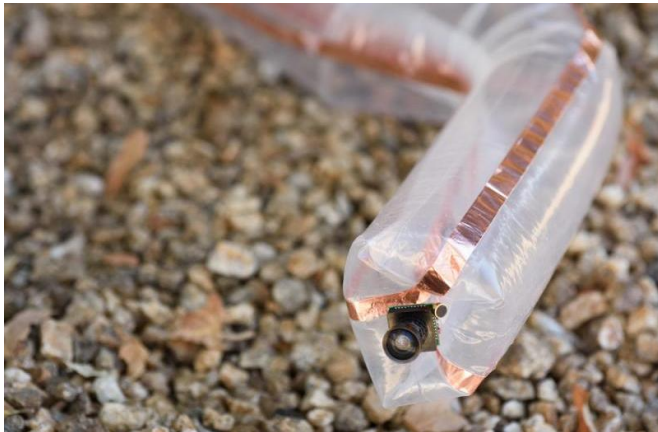
The vinebot is a tube of soft material that grows in one direction. Credit: L.A. Cicero
