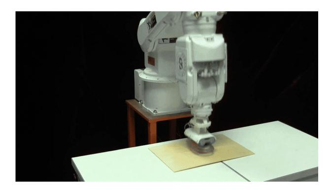
The bioinspired suction disc gripping wood in air. Credit: Wang et al., *Sci. Robot.* 2, eaan8072 (2017)
