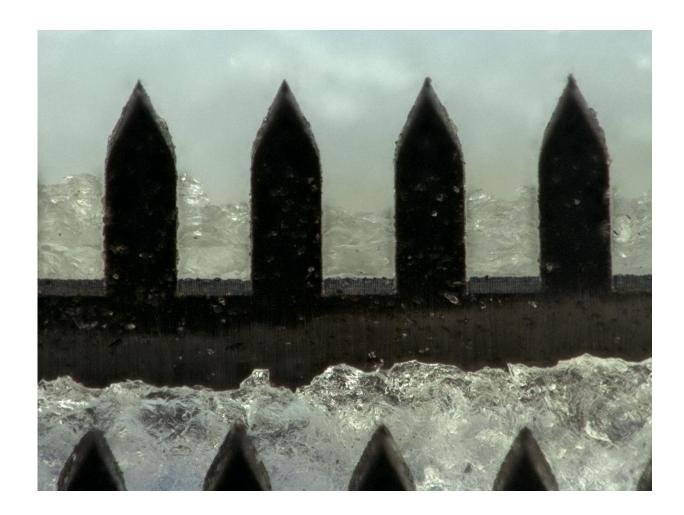
Extreme close-up of the carbon-fiber spinules on the artificial lamellae. Credit: Wang et al., *Sci. Robot.* 2, eaan8072 (2017)
