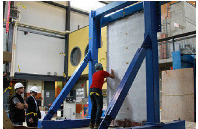
EDCC-reinforced wall being inspected for cracks and damage between earthquake simulation tests. Credit: UBC
