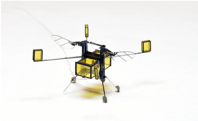
New, hybrid RoboBee can fly, dive into water, swim, propel itself back out of water, and safely land. The RoboBee is retrofitted with four buoyant and a central gas collection chamber. Once the RoboBee swims to the surface, an electrolytic plate in the chamber converts water into oxyhydrogen, a combustible gas fuel. Credit: Yufeng Chen/Harvard SEAS
