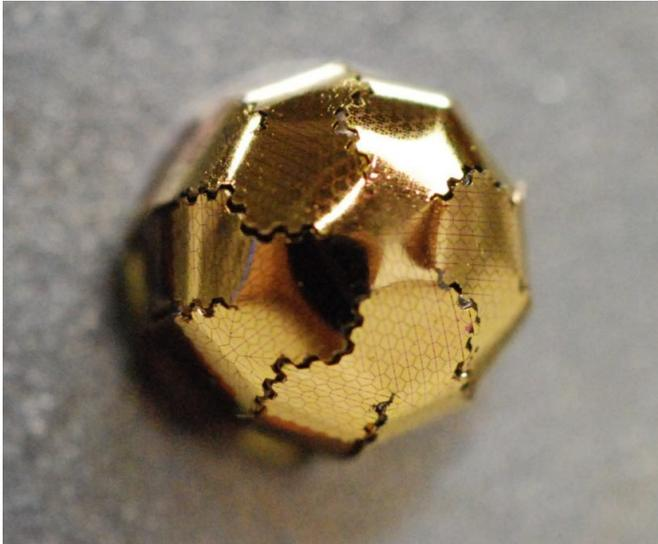
This image shows how the researchers mapped pixels onto the silicon, then cut some sections away so the resulting silicon drapes over a dome shape, with no wrinkles or gaps at the seams. Credit: Yeil Hwan Jung and Kan Zhang.
