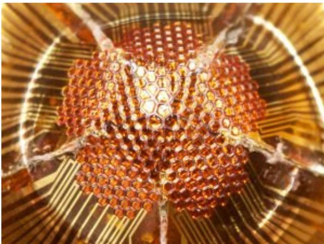
A convex version of the digital image sensor bends like a soccer ball for mimicking an insect's compound eye.
