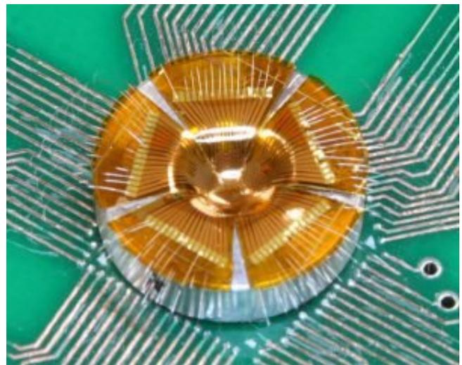
A concave version of the digital image sensor bends inward for creating a hemispherical focal plane array. Credit: Yeil Hwan Jung and Kan Zhang
