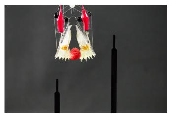
HASEL actuators can be designed as soft grippers to handle and manipulate delicate objects. Credit: Keplinger Lab / University of Colorado Boulder
