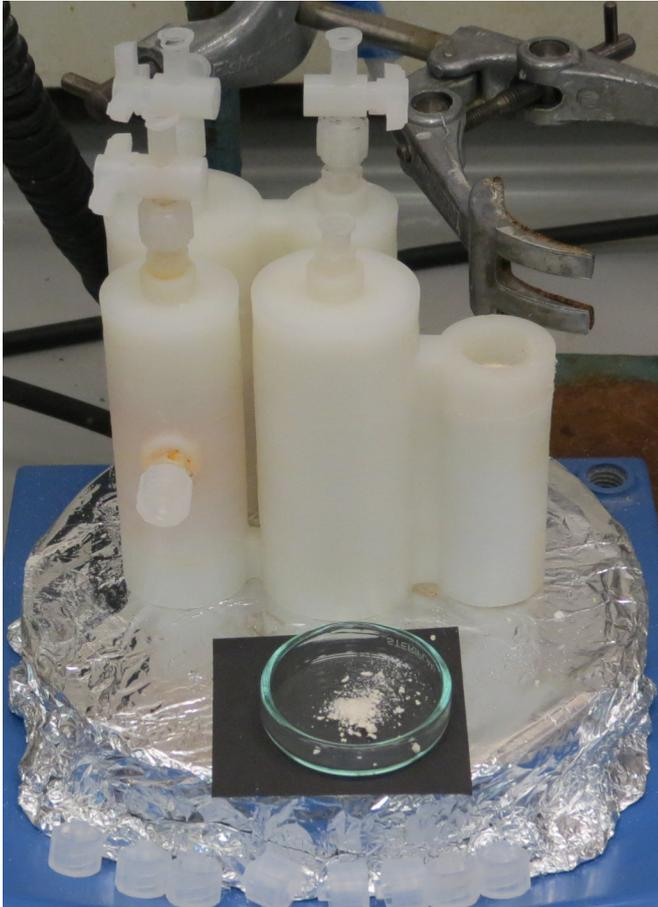
Photograph of the final product of the cartridge synthesis of baclofen with the synthesis cartridge. Credit: Philip J. Kitson and Leroy Cronin
