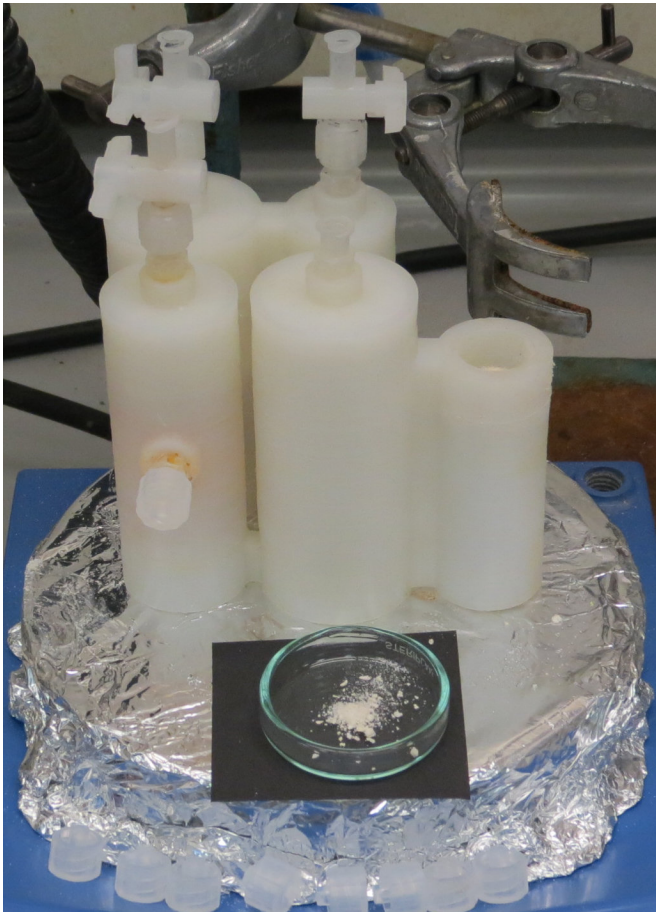
Photograph of the final product of the cartridge synthesis of baclofen with the synthesis cartridge. Credit: Philip J. Kitson and Leroy Cronin
