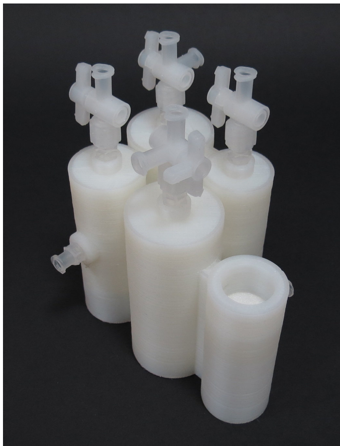
Photograph of the monolithic implementation of the cartridge for the synthesis of baclofen. Credit: Philip J. Kitson and Leroy Cronin
