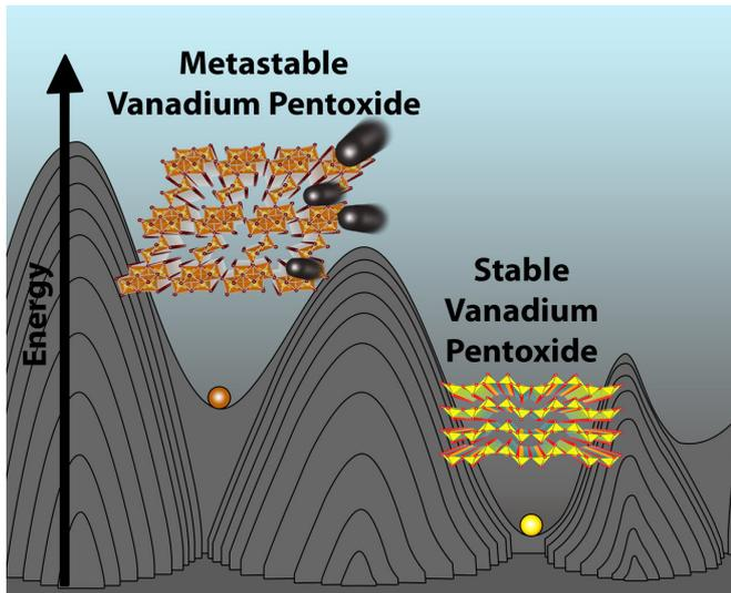
A redesigned metastable phase of vanadium pentoxide ( $V_2O_5$ ) shows extraordinary performance as a cathode material for magnesium batteries. The graphic compares the conventional (right) and metastable structures of  $V_2O_5$ . Credit: Justin Andrews, Texas A&M University
