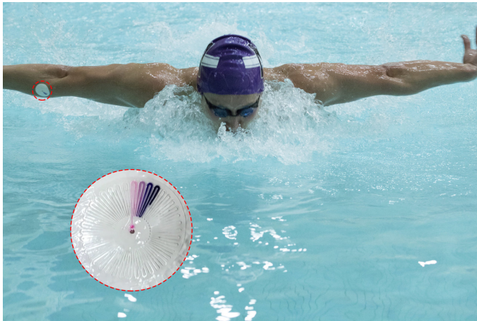
Epifluorescence device measures sweat rate during swimming. Credit: Jonathan T. Reeder (Northwestern University)
