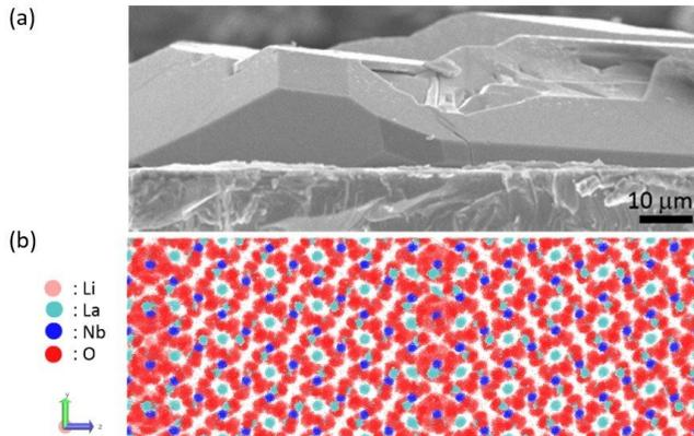
Image (a) is a cross-sectional SEM image of the  $\text{Li}_5\text{La}_3\text{Nb}_2\text{O}_{12}$  crystal layer and image (b) shows computationally simulated trajectories of the Li, La, Nb, and O framework atoms obtained for  $\frac{1}{3}(2-1-1) = (1-21)$  at a temperature of 1300 K. Credit: Nobuyuki Zettsu Ph.D., the Center for Energy and Environmental Science, the Department of Materials Chemistry, Shinshu University.
