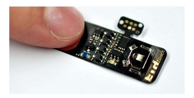
A zero-power receiver for touch communication on a flexible printed circuit board. The circuit board contains all the necessary elements for receiving and demodulating signals as well as energy harvesting by touch. Credit: Michele Magno / ETH Zürich
