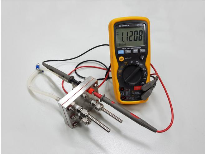
The RMIT-developed proton battery connected to a voltmeter. The working prototype has an energy per unit mass already comparable with commercially-available lithium ion batteries. Credit: RMIT University
