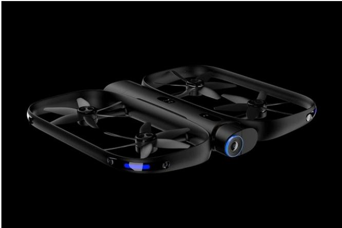
Called R1, Skydio's drone is equipped with 13 cameras that capture omnidirectional video. It launches and lands through an app — or by itself. On the app, the R1 can also be preset to certain filming and flying conditions or be controlled manually. Credit: Skydio
