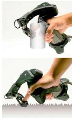
(Left) The CLAW's configuration and components. (Right) The CLAW as it grabs a virtual object, and touches a virtual surface. Credit: Microsoft Research
