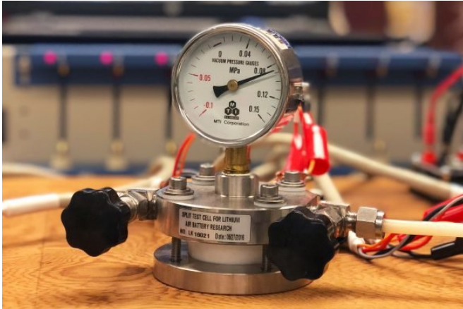
The experimental lithium-air battery. Credit: Amin Salehi-Khojin
