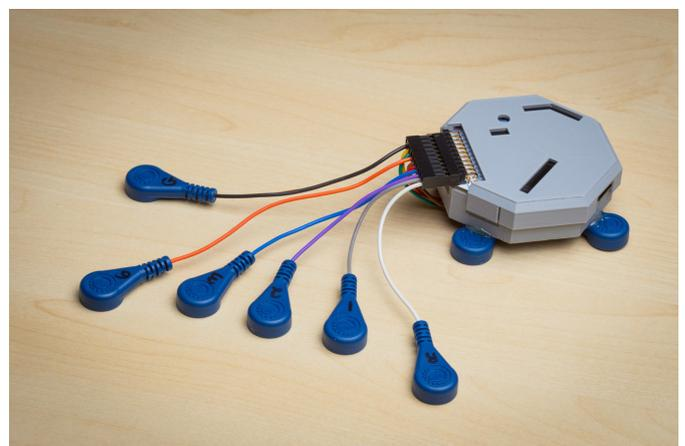
The system is made up of a custom circuit board, a battery and off-the-shelf electrodes encased in a 3-D-printed case. Credit: University of California San Diego
