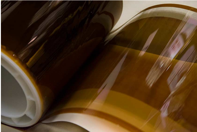
A roll of perovskite film made by the slot-die coating method. Credit: Dennis Schroeder / NREL
