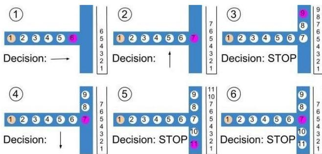
To create a road map, the system starts at a known location and uses a neural network to examine the surrounding area to determine which point is most likely to be the next part on the road. It then adds that point and repeats the process to gradually trace out the road one step at a time. Credit: Massachusetts Institute of Technology
