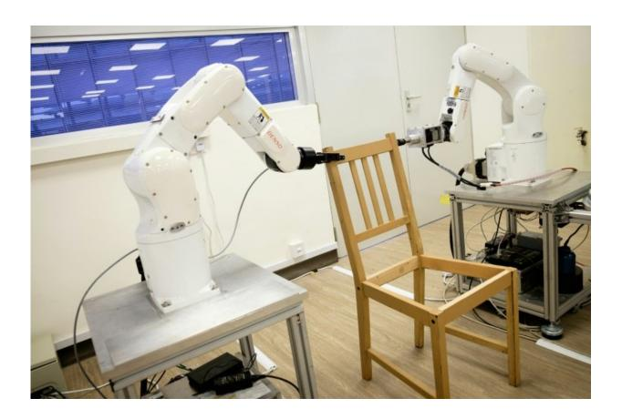
The device, consisting of two mechanical arms with grippers, starts the process by taking photos of the parts spread on the floor with a 3D camera, which is supposed to mimic the cluttered environment after flat-pack furniture is unboxed
