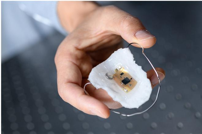
The intraoral electronics with a sodium sensor is based on a breathable elastomeric membrane that resembles a dental retainer. The ultrathin device is flexible and stretchable, and can wirelessly transmit data up to 10 meters. Credit: Rob Felt, Georgia Tech
