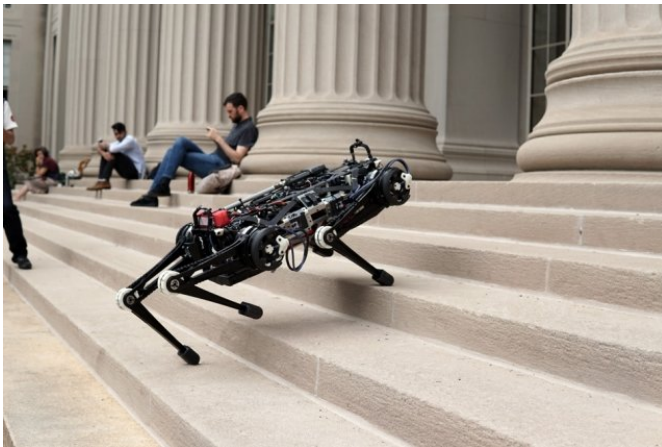
MIT's Cheetah 3 robot can climb stairs and step over obstacles without the help of cameras or visual sensors. Credit: Massachusetts Institute of Technology
