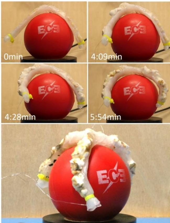
Fiber-reinforced elastomer actuator powered using popcorn wrapped in Nichrome 60 wire. Credit: Steven Ceron et al, Popcorn-Driven Robotic Actuators
