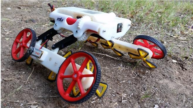
Ben-Gurion University of the Negev researchers designed the Rising Sprawl-Tuned Autonomous Robot (RSTAR) to function simply and reliably, change shape and overcome common obstacles without any external mechanical intervention. RSTAR uses adjustable sprawling legs angled downwards and outwards from its body to creep and crawl and climb over and through a variety of obstacles and surfaces. Credit: Ben-Gurion U
