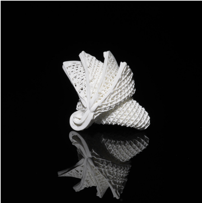
Printed ceramic origami mimicking the Sydney Opera House. Credit: City University of Hong Kong
