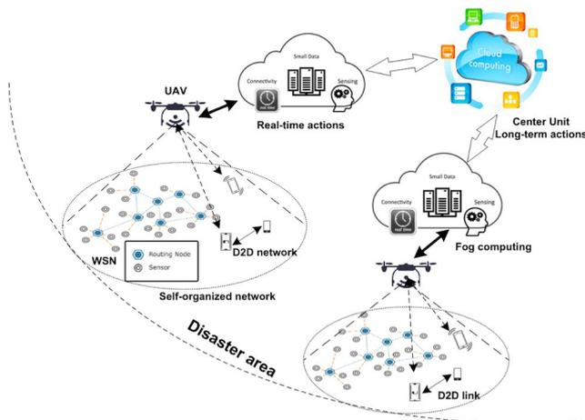
Real-time UAV communications system for disasters scenario. Credit: Duong et al.
