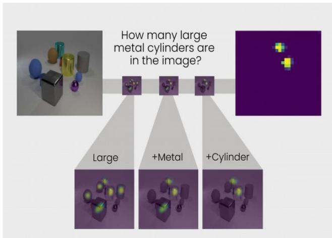
TbD-net solves the visual reasoning problem by breaking it down to a chain of subtasks. The answer to each subtask is shown in heat maps highlighting the objects of interest, allowing analysts to see the network's thought process. Credit: Intelligence and Decision Technologies Group
